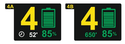
Screen 4B shows the estimated remaining run time, based on the current engine load. The internal electronics measures the average current drain, and every 6s it will calculate how many minutes of driving time remain at this level.
