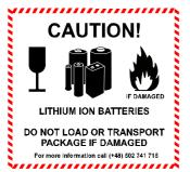
During transportation the battery must be protected against mechanical damage, particularly crushing. Damage of this type poses a fire risk.
