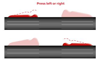
This also means that the propeller will spin as long as the gear is not 0 and at least one button is pressed. This allows for changing the hand that controls the scooter on the way.
