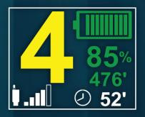
**Current gear** indicates used power level. There are gears 1-9, gear "+" which is a booster gear and "R" – reverse.
